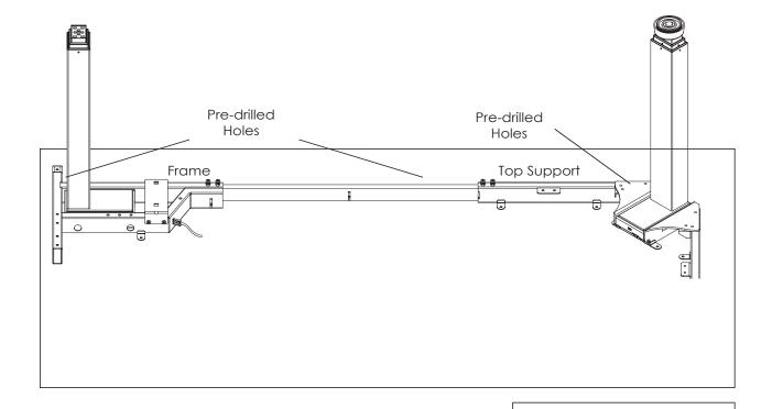
Once the frame is in its final position, attach it to the work surface using the #10 x 5/8" screws (16 total).
